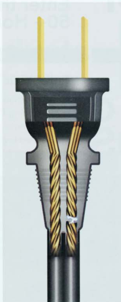
ABOVE: An example of how a typical arc-fault occurs in appliances and other household electrical equipment. PHOTOS COURTESY OF NEMA
